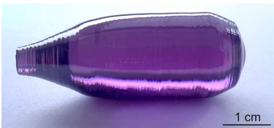
Fig. 3 (La,Nd)(Lu,Sc)O_3 single crystal grown by the Czochralski technique [2].
