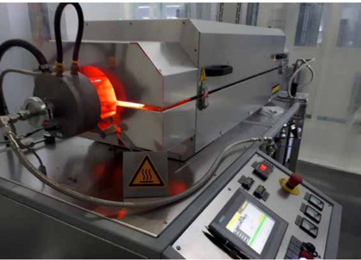
Fig. 1a Reduction equipment in operation for reducing and converting powders into metal bars
