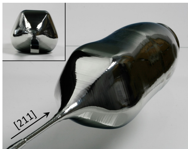
Fig.1 Nicely faceted [211] Ge crystal (45 mm diameter) grown by the Cz technique. The inset figure shows the top view of the crystal, revealing a trapezoid, non-rotational symmetric crystal shape.
