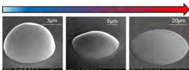
Fig. 3 Influence of deposition temperature: 355 nm indium on molybdenum, deposited at 0.9 Å/s with increasing temperature from left to right: T_{min} (left): ca. 300°C; T_{max} (right): ca. 330°C.
