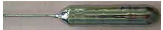
Fig.5 Highly compensated p-type Ga and Sb co-doped \langle 100 \rangle Ge crystal grown for use as photoconductive Ge detectors
