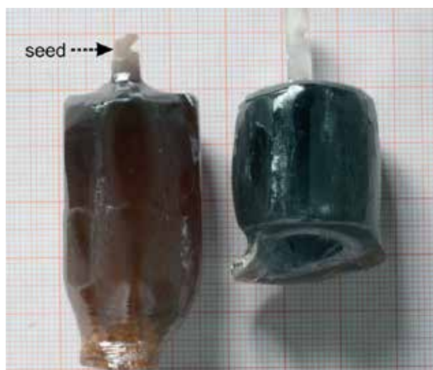
Fig. 1 \text{SrTiO}_3 crystals grown by TSSG (starting temperature 1740^\circ\text{C} ) in an oxygen enriched argon atmosphere (left crystal) and in pure argon (right crystal). All other growth conditions were kept identical. Note the spiral formation and bluish coloration of the right crystal. From Ref. [6] reproduced by permission of The Royal Society of Chemistry (RSC).
