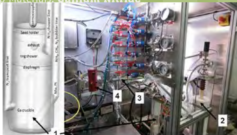
Fig. 1 QuartzGaN equipment with reactor scheme (1), HCN reactor (2), gas cell for FTIR (3) and MCT detector (4)
